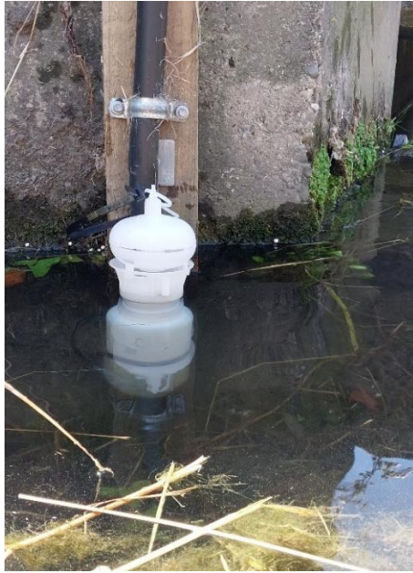
Figure 4: Rain Event Sampling Bottle
