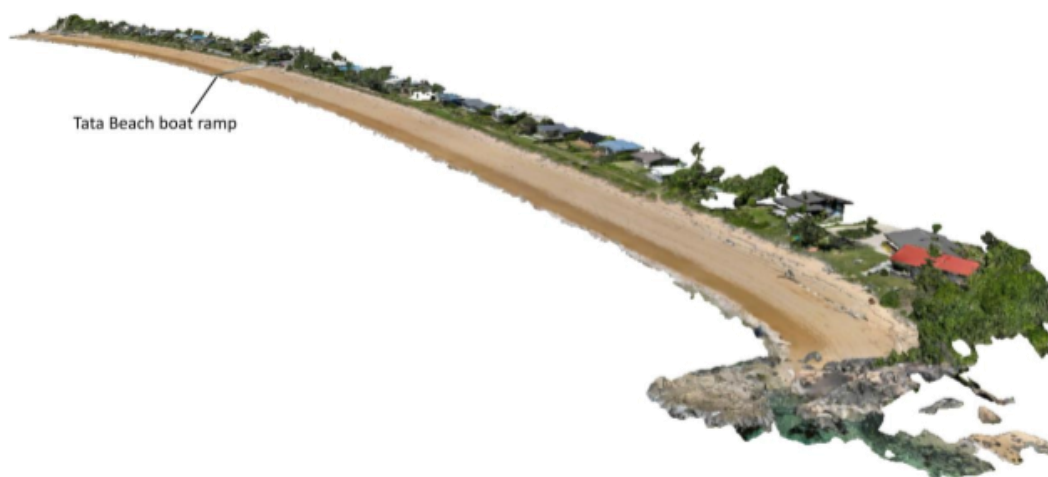
Figure 4: Oblique view of the 3D model of Tata Beach produced from the drone survey flown in December 2025. The view is looking roughly to the northeast from the southwestern end of the beach. The Tata Beach boat ramp is visible part-way along the beach.
