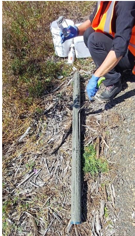
Figure 8 Taking sediment samples from the jellyfish membrane cartridge
