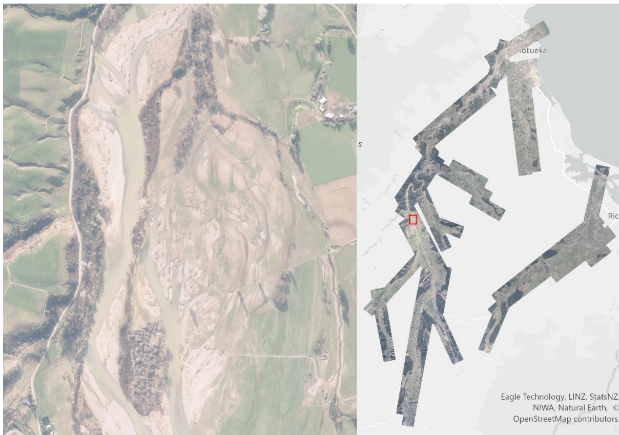
Figure 7: (left) An example of the Aerial Surveys orthophotography taken near Hinetai on the Upper Motueka River; (right) Full extent of the aerial photography captured on 17 July 2025. The area shown on the left is indicated in red.
