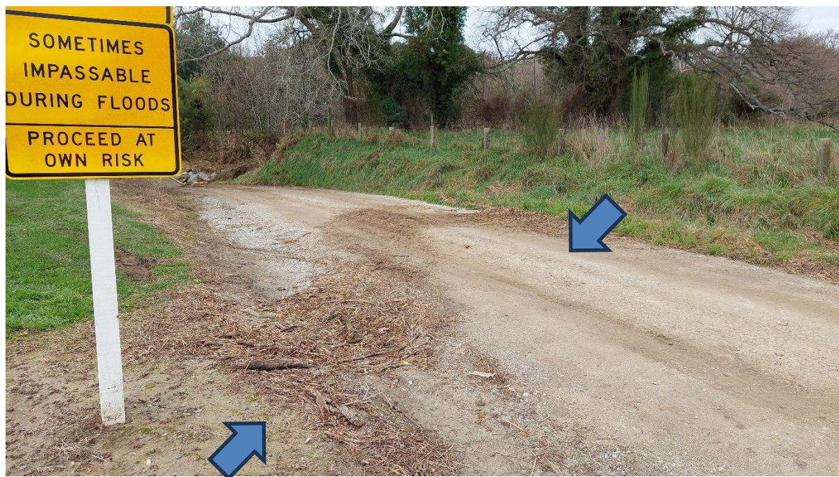
Figure 9: Example of a debris line surveyed by the Natural Hazards team in the Moutere valley at the Holaway Road ford. The two ends of the debris line are indicated with arrows.
