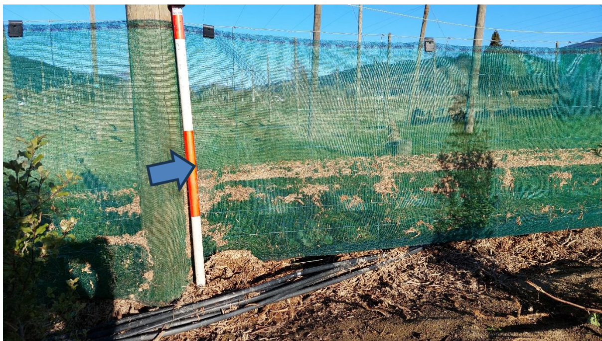
Figure 10: Example of a 'seed line' surveyed by the Natural Hazards team at Old School Road near Kohatu after the 27 June flood event. The 'seed line' (arrowed) records the flood level through fine debris caught on fencing material.
