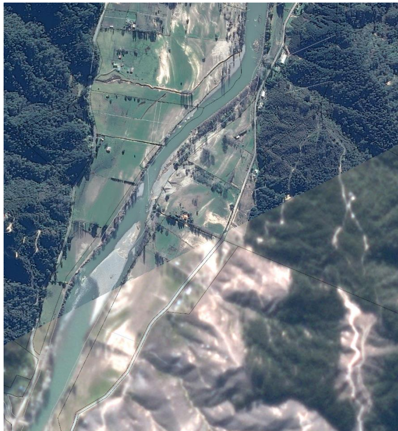
Figure 16: Comparison of different satellite imagery available through the disaster charter: (top) Pleiades 0.7 m resolution imagery; (bottom) PlanetScope 3 m resolution imagery.
