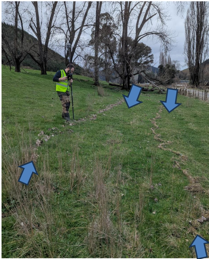
Figure 12: Hamish Sutton from NIWA surveying debris lines in the Motueka valley near Woodstock after the July flood event. The line on the left is from the 27 June flood event, while the line on the right is from the 11 July flood event.
