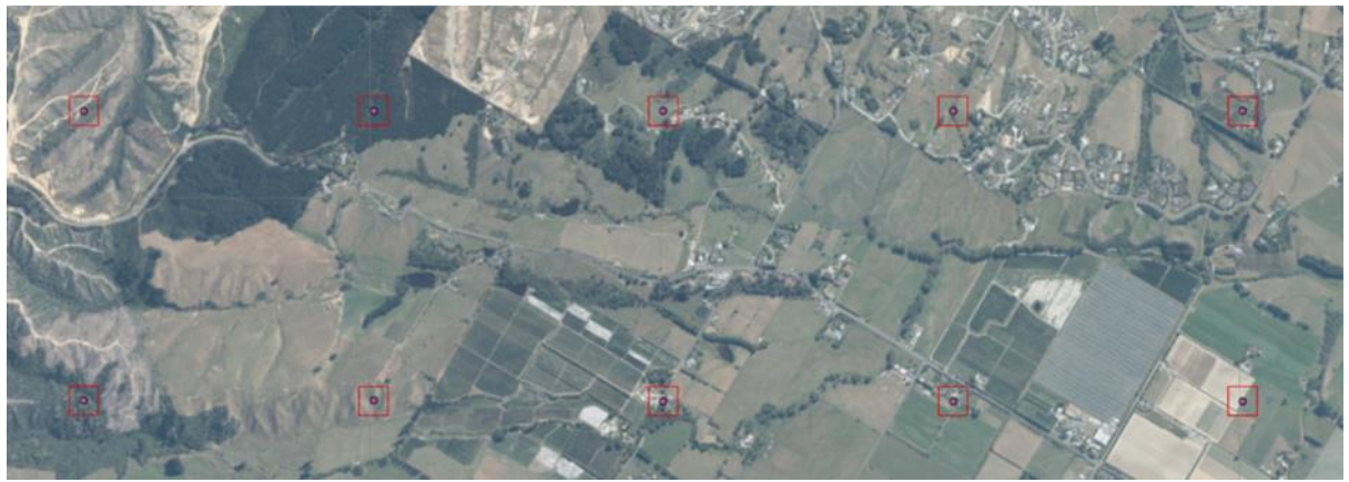
Figure 15: Grid-based point sampling
