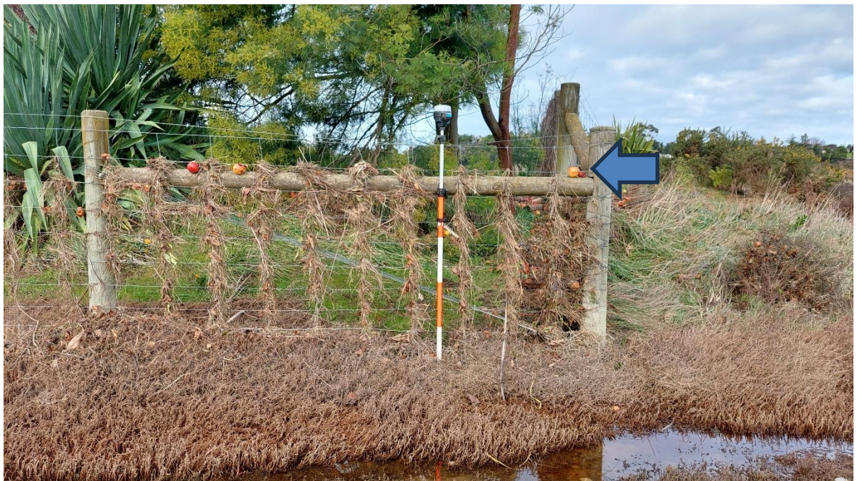
Figure 11: Example of debris caught in a fence surveyed by the Natural Hazards team on Batchelor Ford Road in the lower Moutere valley after the 27 June flood event. The arrow indicates the maximum level of debris caught on the fence.
