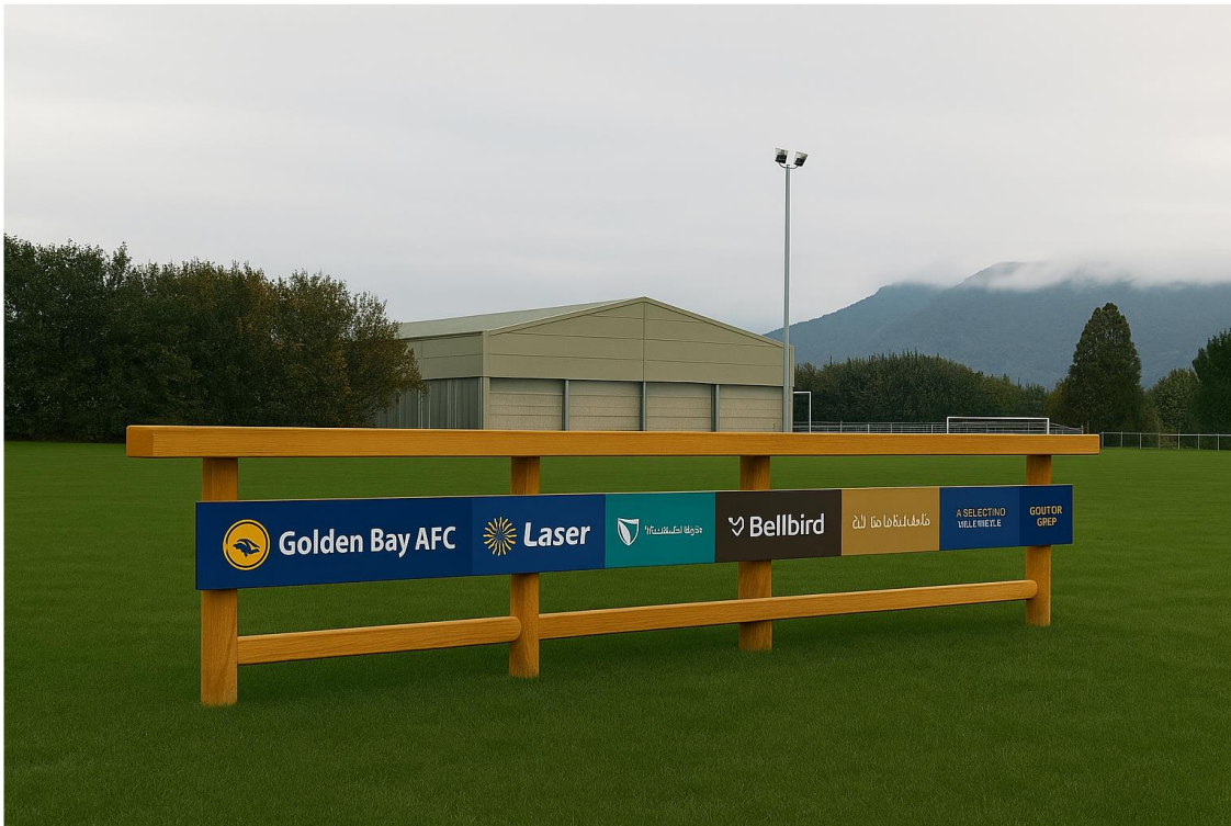
Image 5: AI generated example of Barrier leaner - The leaner dimensions: 600mm sign, so 800mm high total. And seat plank on top width 200mm.
