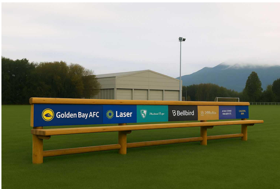
Image 4: AI generated example of seating plan - not to measurement. On Junior Field. Seat height: 450mm, with a back of 600mm which is the sign size, width total 600mm, Length 30m, with gaps for ease of fetching rouge balls.
