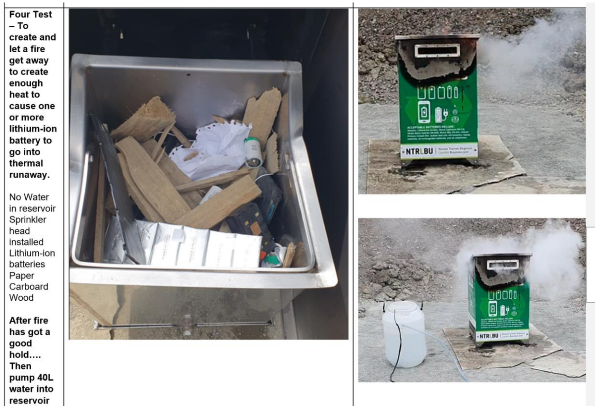
Figure 1: Pictures showing test 4 – allowing fire to get established and then demonstrate that the fire suppression systems can put it out.
