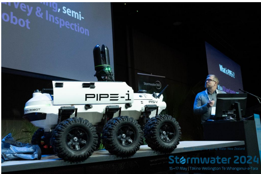
Figure 8: Pipe inspection robot developed by Becca
